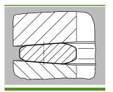
high-temperature gaskets with flanges with raised or flat face flanges. The gaskets are then centred on the bolts. Profile H15, with a loose centring ring, is ideal for use with gaseous media and/or centring ring with widths greater than 15 mm. Profiles H7, H9 and H15 have an osculating radius
